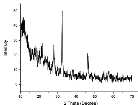
**Fig.6: X-ray diffractogram of AgNPs.**
