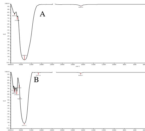
Fig.2:FT-IR spectrum of leaf extract of (a), Silver nano particle (b)
