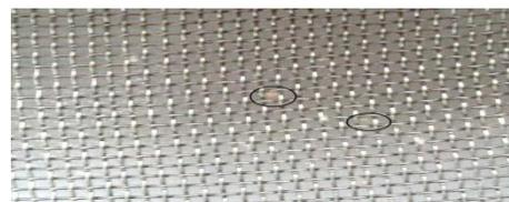
**Fig. 4: Sieve No. 22 (enlarged view), Brand C**
