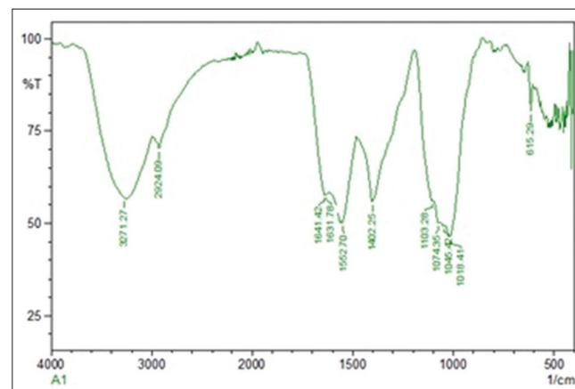
Fig. 1: Fourier transform infrared spectroscopy spectrum of biosynthesized titanium dioxide nanoparticles
