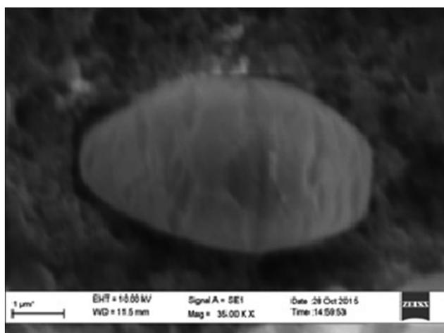
Fig. 2: Scanning electron microscopy image of the biosynthesized titanium dioxide nanoparticles
