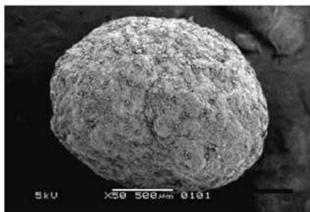
Fig.2: Scanning electron microscopic image of Doxofylline loaded Microbeads at 5kV.
