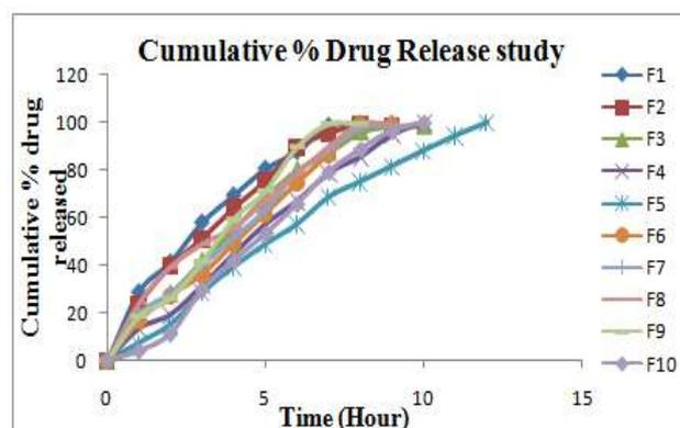
Fig.4: Showing in vitro drug release study of Doxofylline loaded microbeads.
