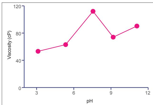
Fig. 3: Effect of pH on viscosity of 20% w/v shea gum mucilage at 25°C and shear rate of 1 rpm
