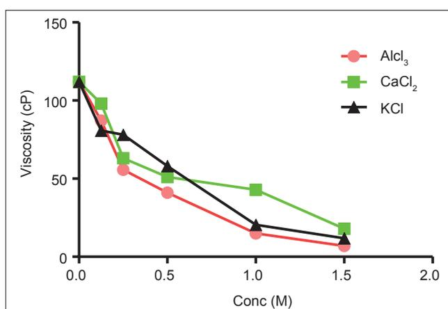
Fig. 4: Effect of electrolyte concentration on viscosity of 20% w/v shea gum mucilage determined at 27°C and shear rate of 1 rpm
