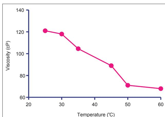
Fig. 2: Effect of temperature on the viscosity of 20% w/v shea gum mucilage at shear rate of 1 rpm
