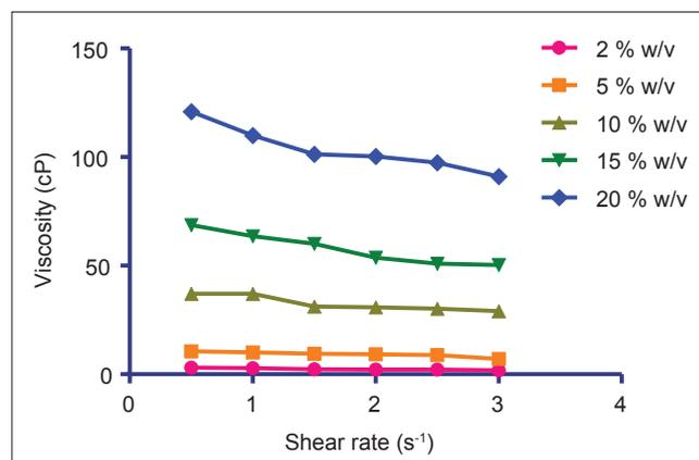
Fig. 1: Flow curves of different concentrations of purified shea gum at 25°C
