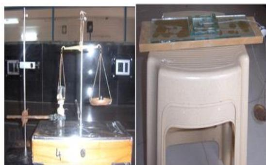
Fig IV (a) and V (a): Instruments for determination of ex-vivo Mucoadhesion and peel adhesion strengths
