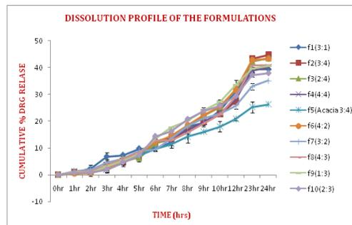
**Fig II: Dissolution Profile of the Formulations**
