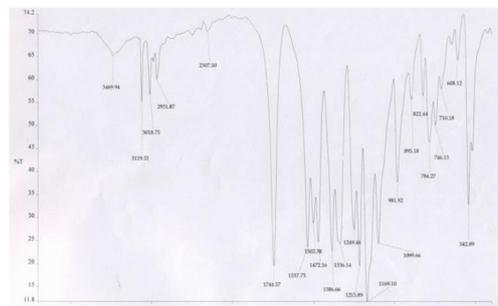
Fig X (a): IR Spectrum of Satranidazole
