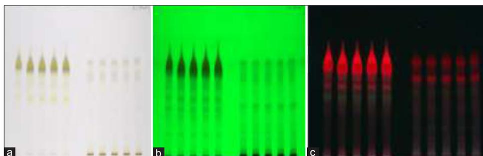
**Fig. 1: High-performance thin layer chromatography fingerprint profile of phytosterols of leaf extract of *Holooptelea integrifolia* (Roxb.) Planch (Track 1-5: Petroleum ether extract, Track 7-11: Methanol extract, Note: There were no data available for track 6). (a) HPTLC plate seen at visible light. (b) HPTLC plate seen at 254 nm. (c) HPTLC plate seen at 366 nm**
