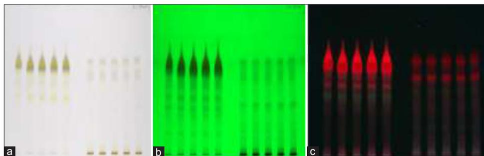
**Fig. 1: High-performance thin layer chromatography fingerprint profile of phytosterols of leaf extract of *Holoptelea integrifolia* (Roxb.) Planch (Track 1-5: Petroleum ether extract, Track 7-11: Methanol extract, Note: There were no data available for track 6). (a) HPTLC plate seen at visible light. (b) HPTLC plate seen at 254 nm. (c) HPTLC plate seen at 366 nm**
