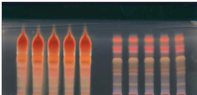
**Fig. 2: Fingerprint analysis of phytosterols of *Holoptelea integrifolia* (Roxb.) Planch leaves after derivatization with anisaldehyde sulfuric acid reagent inflorescence at 366 nm**
