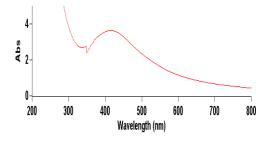
Fig.2:UV-Visible spectra of synthesized silver nanoparticles
