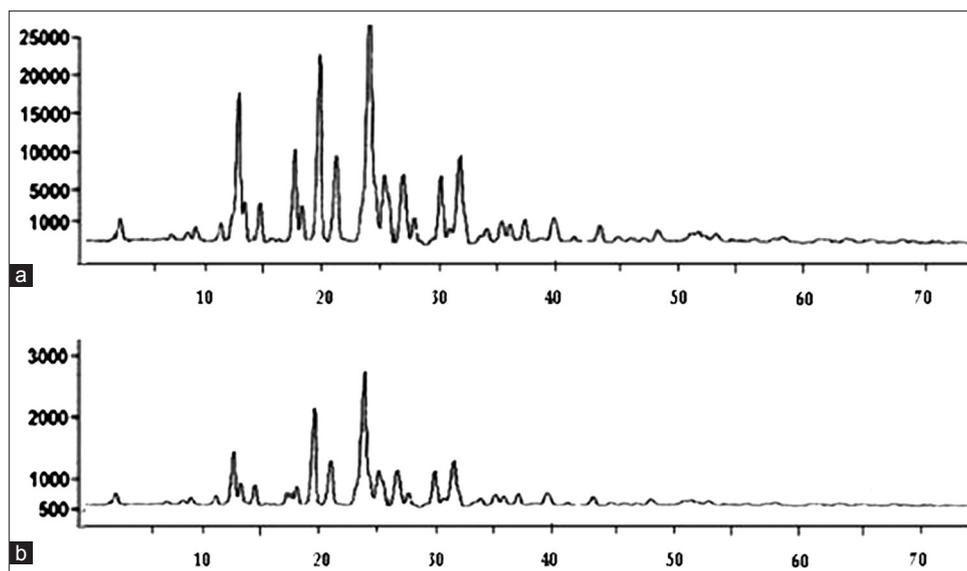
Fig. 8: X-ray diffraction pattern of (a) valsartan (b) lquisolid compact
