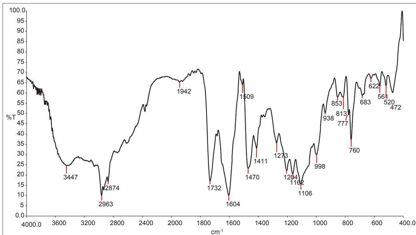
Fig.2: Infrared spectra of valsartan liquisolid compact
