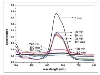
Fig. 4: Variation of dye concentration with time reduction in ultraviolet-visible absorption peaks with time
