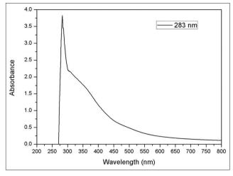
Fig. 1: Ultraviolet-visible absorption spectrum of Iron oxide nanoparticle
