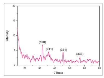
Fig. 3: X-ray diffractometer pattern of Iron oxide nanoparticle
