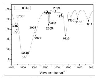
Fig. 2: Fourier transform infrared spectroscopy spectrum of Iron oxide nanoparticle
