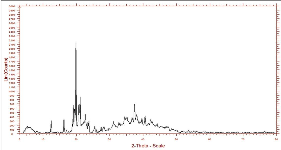
Fig. 6: Powered X-ray diffractometry of optimized formulation
