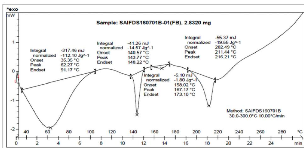
Fig. 4: Differential scanning calorimetry thermogram of optimized formulation
