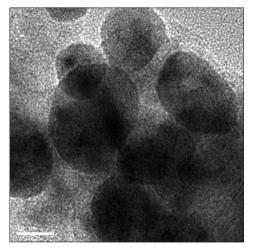
Fig. 6: Transmission electron microscopic image of *Camellia* sinensis extract-mediated synthesized copper nanoparticles at 10 nm scale
