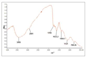
Fig. 8: Fourier transform infrared spectroscopy spectra of copper nanoparticles synthesized using *Camellia sinensis* leaf extract
