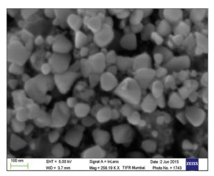
Fig. 5: Scanning electron microscopy image of *Camellia* sinensis extract-mediated synthesized copper nanoparticles at 100 nm scale
