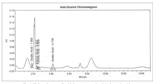
Fig. 1: High-performance liquid chromatogram (peaks) of organic acids
