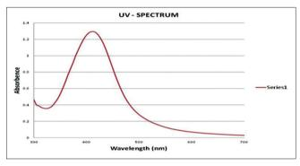
Fig. 3: Ultra violet-visible spectra of silver nanoparticles synthesized by leaf callus extract
