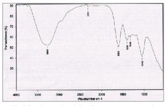
Fig. 7: Fourier transform infrared spectroscopy spectra of stabilized silver nanoparticles
