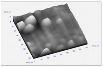
Fig. 6: Atomic force microscope image of silver nanoparticles
