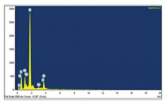
Fig. 5: EDS pattern of silver nanoparticles
