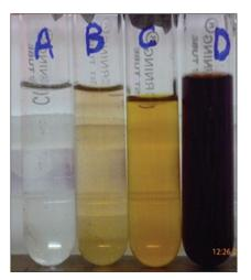
Fig. 2: Rapid color change of AgNO<sub>3</sub>; A (0-5) B (5-10) C (10-15) minutes D (2 hrs)
