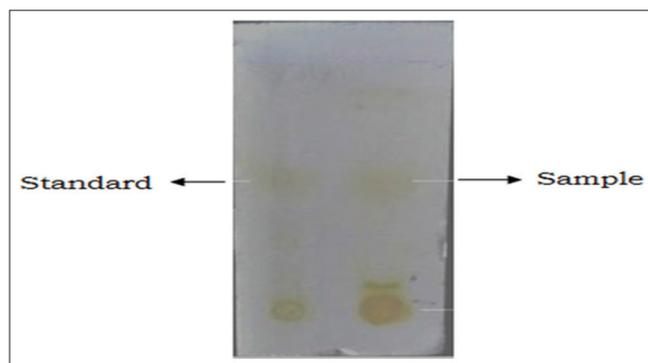
**Fig. 1: Thin layer chromatographic analysis of isolated compound from Chrozophora plicata leaves and its comparison with standard flavonoid kaempferol**
