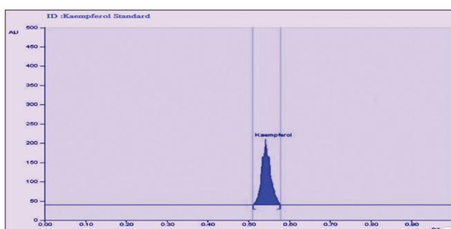
Fig. 7: Kaempferol standard peak densitogram display (scanned at 254 nm)
