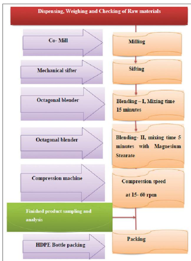
Fig. 2: Process flow chart during manufacturing process of antihypertensive tablets
