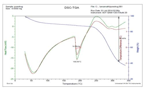
Fig. 5: Differential scanning calorimetry thermal analysis of levosulpiride
