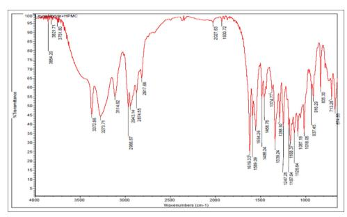
Fig. 2: Fourier transform infrared spectrum of levosulpiride with chitosan
