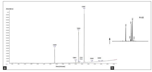
Fig. 1. (a) Gas chromatography mass spectrometer (GC/MS) analysis of methyl esters fatty acids (FAME) present in corn oil sample from Ecuador. (b) Analysis of FAME present in corn oil described for Lantos *et al.*, 2015 [10]
