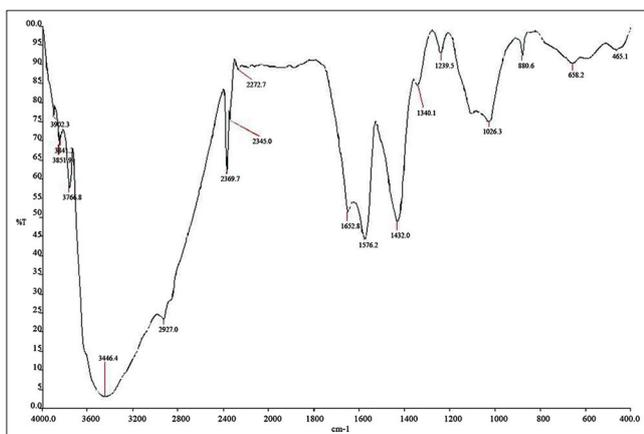
**Fig. 2: Fourier transform infrared spectroscopy image of chitosan**
