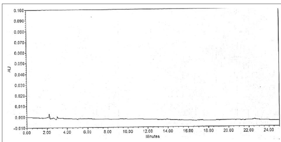
Fig. 2: Typical chromatogram of blank
