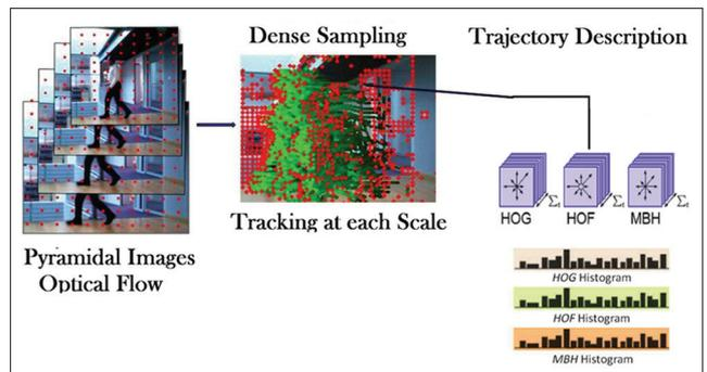
Fig. 6: Sample illustration of a basic space time trajectory approach for action recognition
