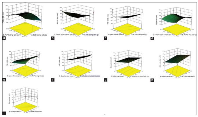
Figure 2: 3D plots for effect of SLS to CRM ratio, PVP K60 to CRM ratio, solvent to antisolvent ratio, and speed of mixing on particle size distribution [i.e. PSD d (90)] (a-f) and zeta potential (g-i)
