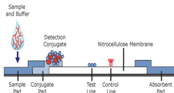
Fig. 2: Diagram of the lateral flow immunoassay (Reproduced from: web)
