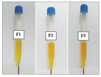
Fig. 3: Centrifugation result of red palm olein nanoemulsion
