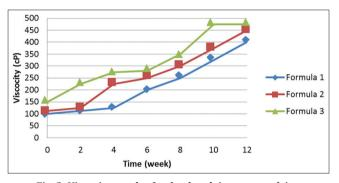
Fig. 2: Viscosity result of red palm olein nanoemulsion
