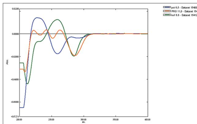
**Fig. 4: First derivative spectra were calculated with  $\Delta\lambda$  8 nm**
