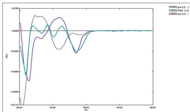
**Fig. 2: First derivative spectra were calculated with  $\Delta\lambda$  2 nm**
