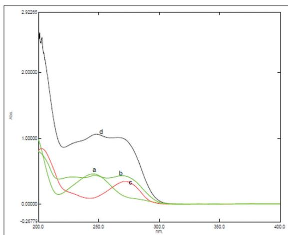
**Fig. 1. Absorption spectra of (a) 6.5 µg/mL paracetamol, (b) 11.0 µg/mL propyphenazone, (c) 6.6 µg/mL caffeine, (d) the ternary mixture**
