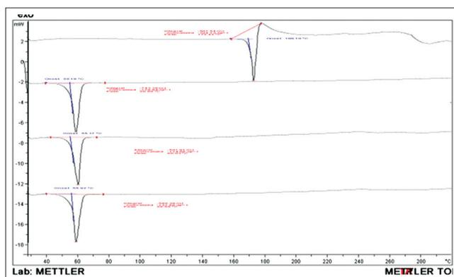
Fig. 5: Differential scanning calorimetry thermo grams of candesartan cilexetil (a), polyethylene glycol 6000 (b), solid dispersion (SD) 1:2 (c) and SD1:4 (d)
