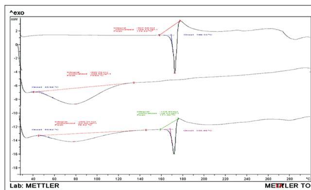
Fig. 6: Differential scanning calorimetry thermo grams of candesartan cilexetil (a), hydroxypropyl-β cyclodextrin (b) and inclusion complex 1:1 (c)
