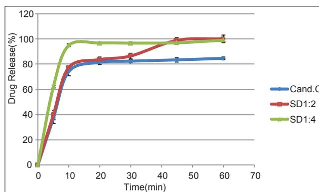
Fig. 8: Dissolution profile of candesartan cilexetil from pure drug, solid dispersion (SD) 1:2 and SD1:4 (weight ratio)
