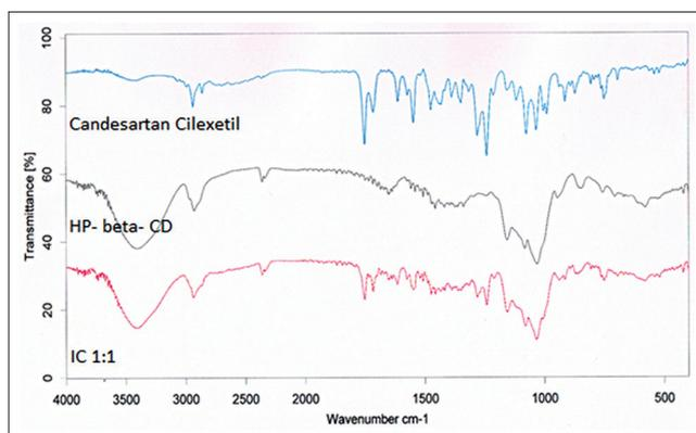
Fig. 3: Fourier transforms infrared spectra of candesartan cilexetil, hydroxypropyl-β cyclodextrin and inclusion complexes 1:1
