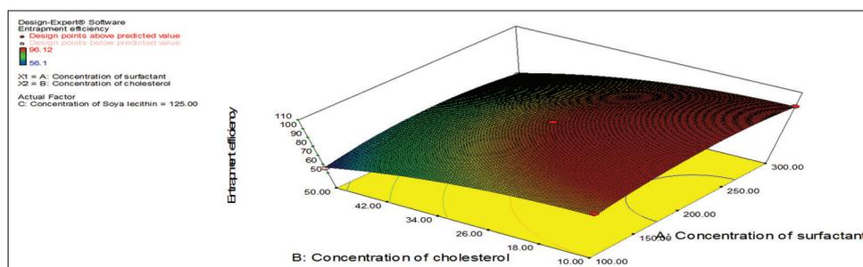
Fig. 7: Response surface plots showing the interactions between the concentration of surfactant and concentration of cholesterol on entrapment efficiency
