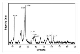
Fig. 2: X-ray diffraction analysis of nanoclay
