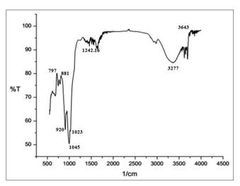
Fig. 7: Fourier transform-infrared analysis for organobentonite
