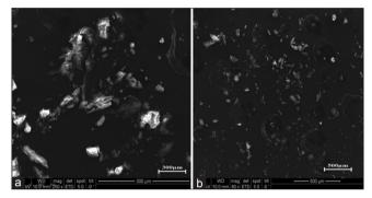
Fig. 3: (a and b) Scanning electron microscopy images of nanoclay before hydrogen peroxide treatment
