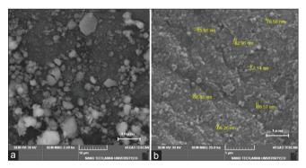
Fig. 4: (a and b) Scanning electron microscopy images of nanoclay after hydrogen peroxide treatment
