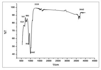
Fig. 5: Fourier transform-infrared analysis for nanoclay
