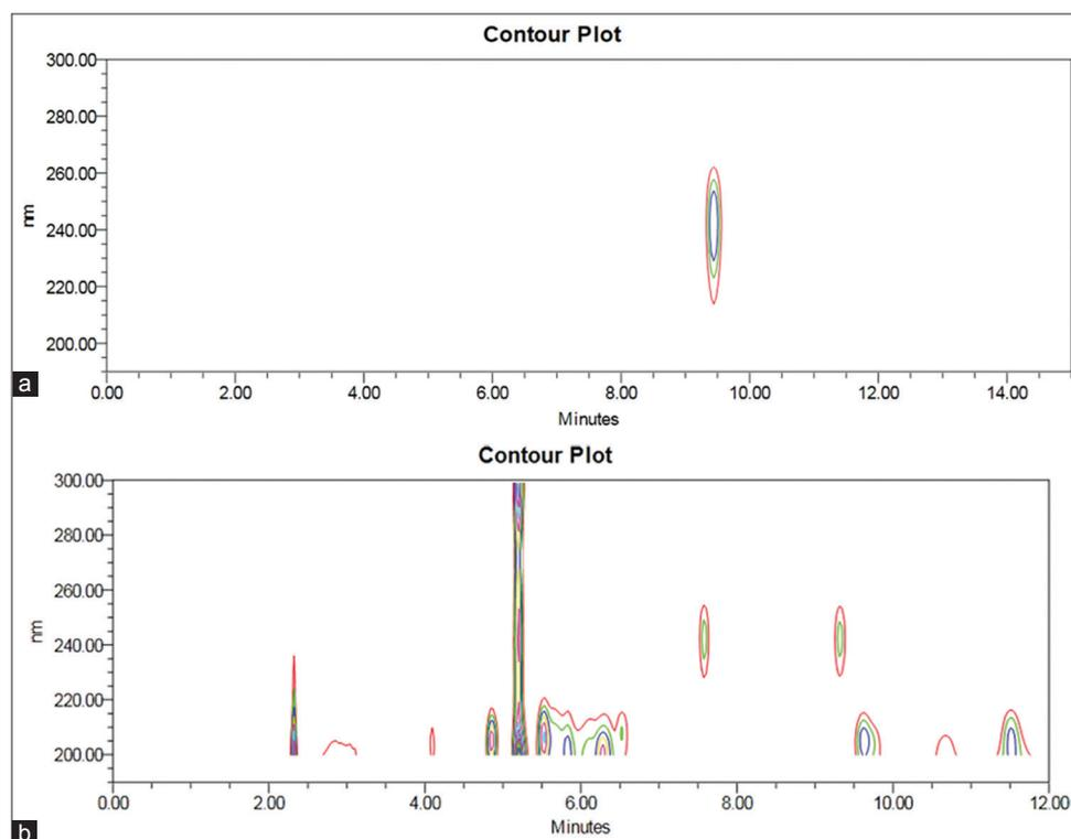
Fig. 3 (a) Contour of guggulsterone (GZ) in standard solution. (b) Contour of GZ in chloroform extract of *Gokshuradi Guggulu*
