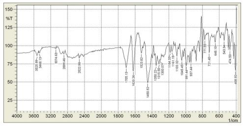
Fig. 2: Infrared spectra for pure moxifloxacin
