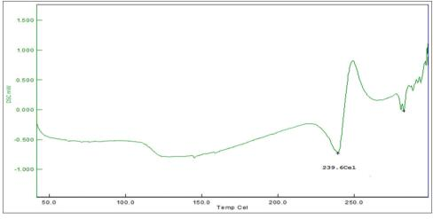
Fig. 3: Differential scanning calorimetric of hydrochloride
