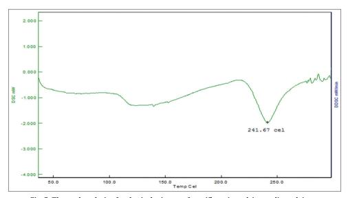
Fig. 5: Thermal analysis of a physical mixture of moxifloxacin+gelrite+sodium alginate
