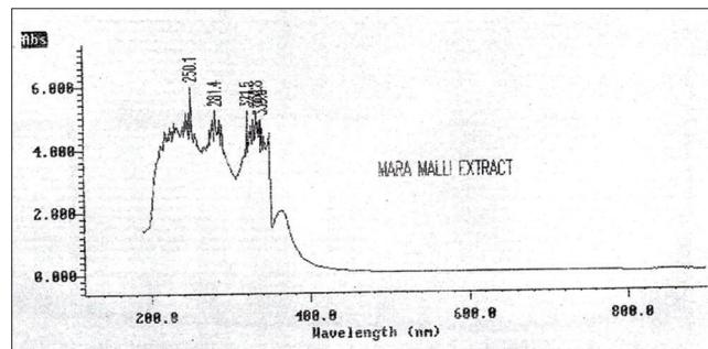
**Fig. 1:** Absorption spectrum of purified compound from *Millingtonia hortensis* (A peak at around 210 nm is indicating the presence of a peptide bond in the compound)
