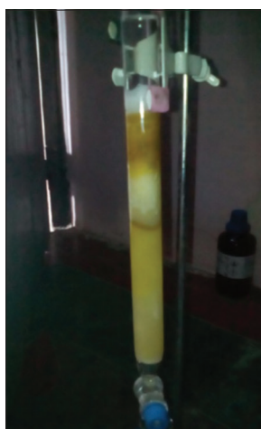
Fig. 2: Isolation of antioxidant by column chromatography
