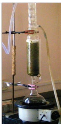
Fig. 1: Extraction by Soxhlet method
