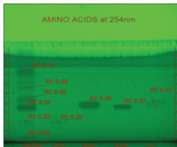
Fig. 5: High-performance thin-layer chromatography chromatogram of the amino acid at 254 nm
