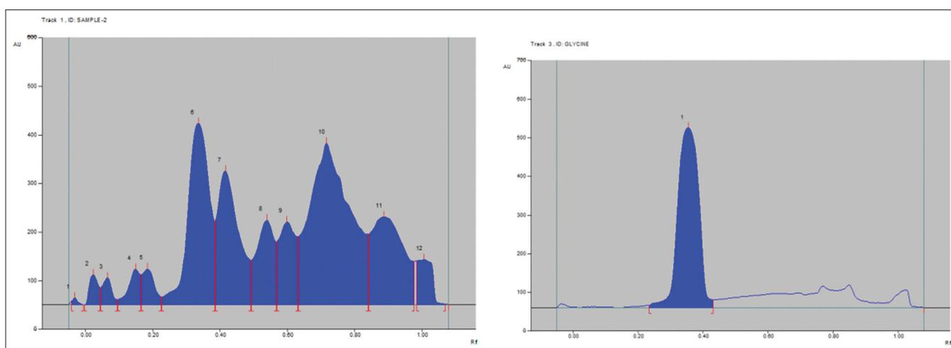
Fig. 7: Comparison of high-performance thin-layer chromatography fingerprint sample with standard amino acid (glycine)
