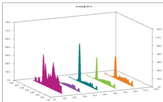
Fig. 3: 3- Dimensional view of chromatogram of sample with four standard amino acids
