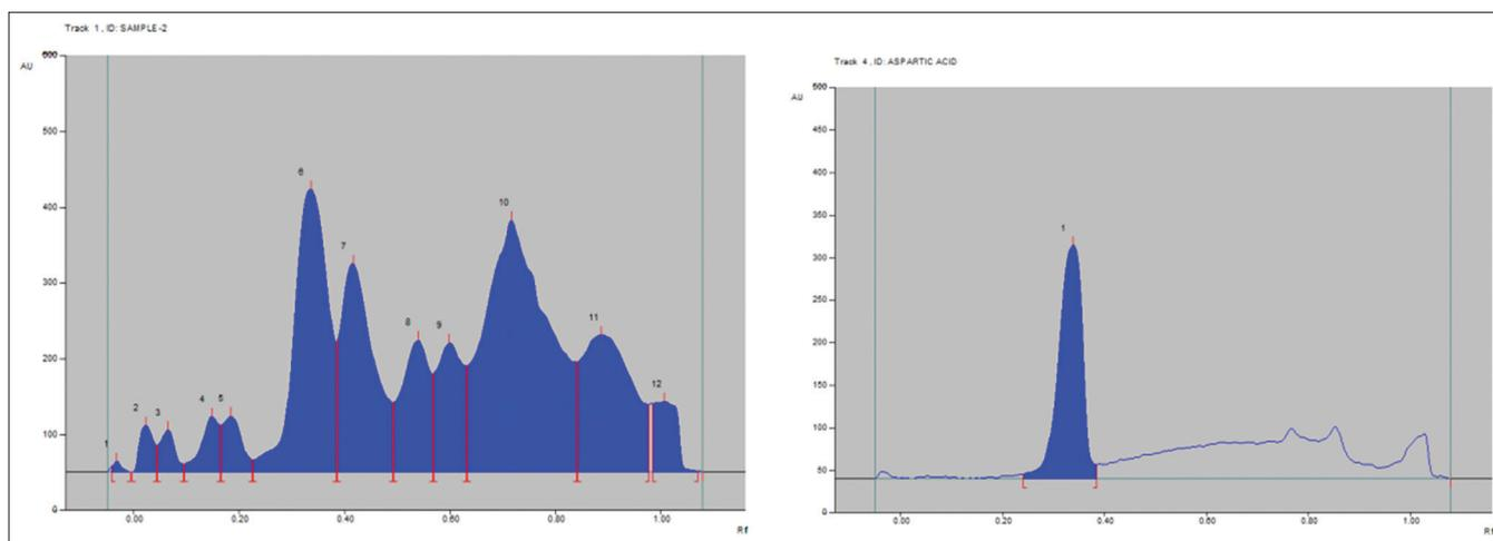
Fig. 6: Comparison of high-performance thin-layer chromatography fingerprint sample with standard amino acid (aspartic acid)
