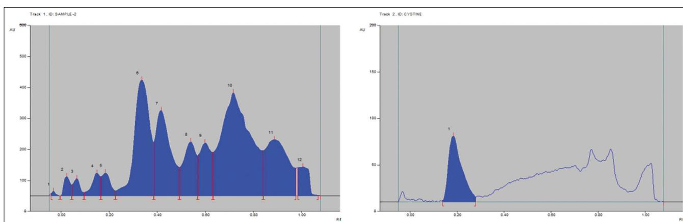
Fig. 8: Comparison of high-performance thin-layer chromatography fingerprint sample with standard amino acid (cysteine)
