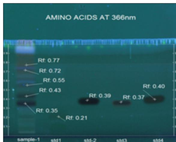
Fig. 4: High-performance thin-layer chromatography chromatogram of the amino acid at 366 nm
