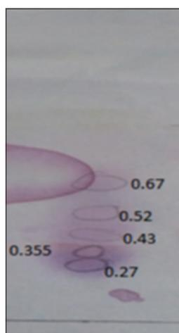
Fig. 2: Paper chromatography of isolated amino acid detected using ninhydrin
