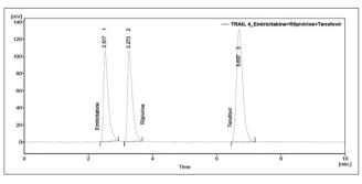
Fig. 2: Optimized chromatogram of emtricitabine, rilpivirine, and tenofovir alafenamide
