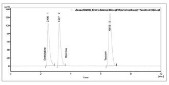
Fig. 3: Assay chromatogram of emtricitabine, rilpivirine, and tenofovir alafenamide
