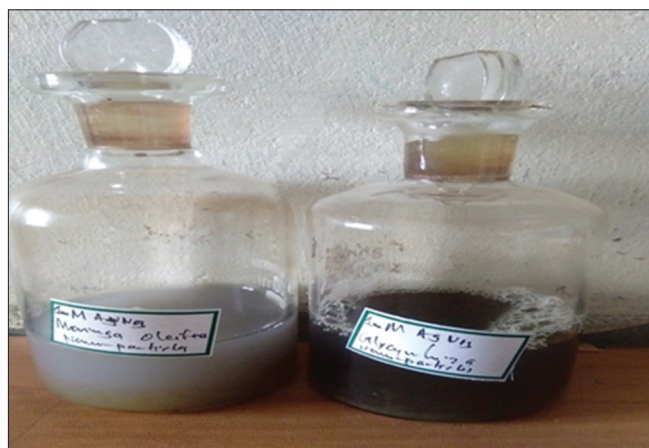
Fig. 2: Synthesized silver nanoparticles using Moringa oleifera seed extract and Glycyrrhiza glabra stem extract
