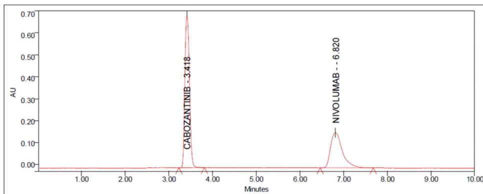
Fig 2: Typical standard chromatogram for carbozantinib and nivolumab
