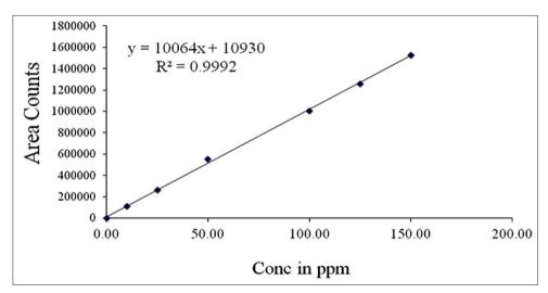
Fig. 4: Linearity plot for rilpivirine
