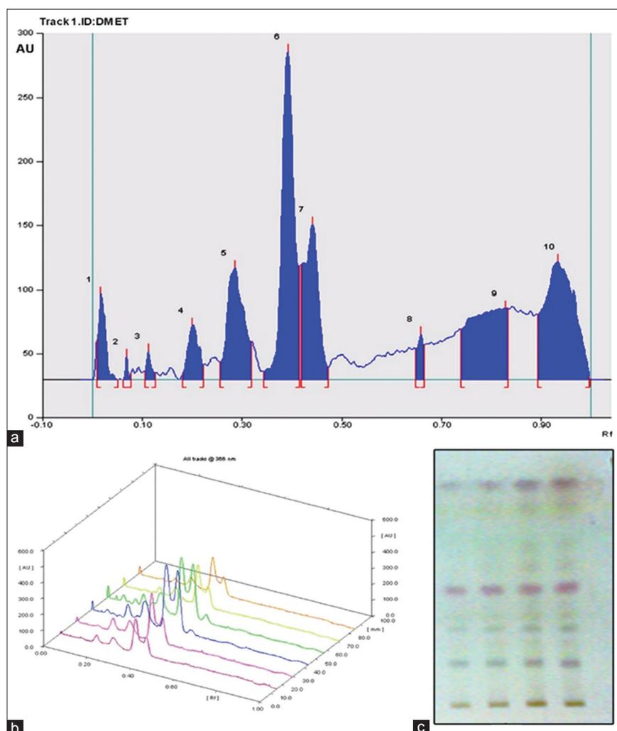
Fig. 2: High-performance thin-layer chromatography chromatogram of an ethanolic extract of *Diospyros montana* (Roxb.) leaves. a) HPTLC finger printing of ethanolic extract of *D. montana* leaves, b) HPTLC three-dimensional evaluation, c) HPTLC photo documentation of ethanolic extract of *D. montana* leaves
