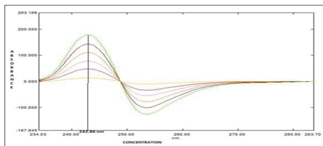
Fig. 7: Ratio first derivative absorption spectra of DAPO (2-12 µg/ml)
