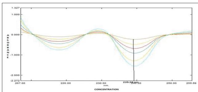
Fig. 8: Ratio first derivative absorption spectra of sildenafil citrate (10-60 µg/ml)
