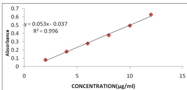
Fig. 4: Calibration curve data for dapoxetine hydrochloride standard
