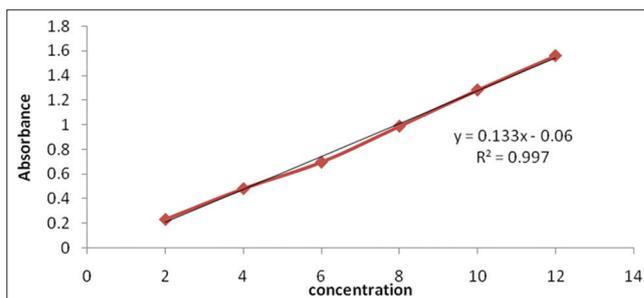
Fig. 9: Calibration curve of dapoxetine hydrochloride
