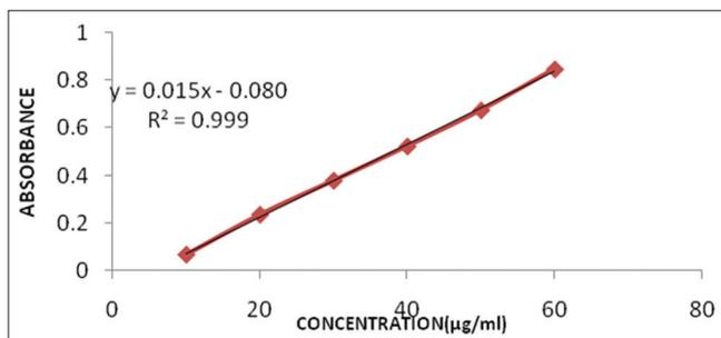
Fig. 3: Calibration curve data for sildenafil citrate standard
