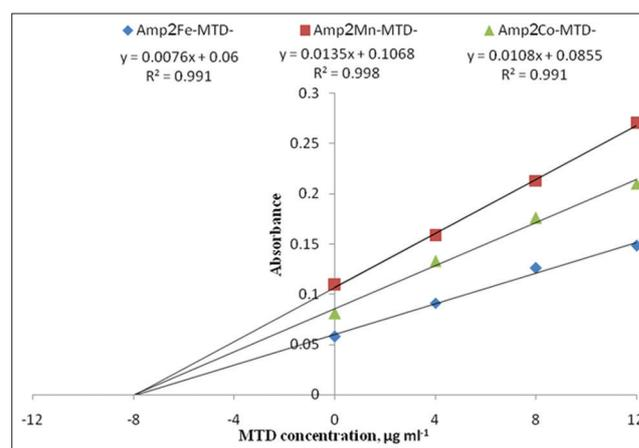
Fig. 7: Standard additions method for assay of Aldosam
