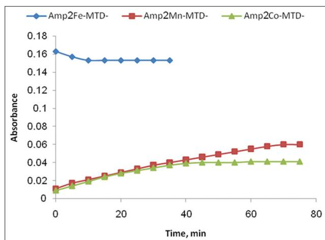
Fig. 4: Effect of the stability time on the formed ternary complexes
