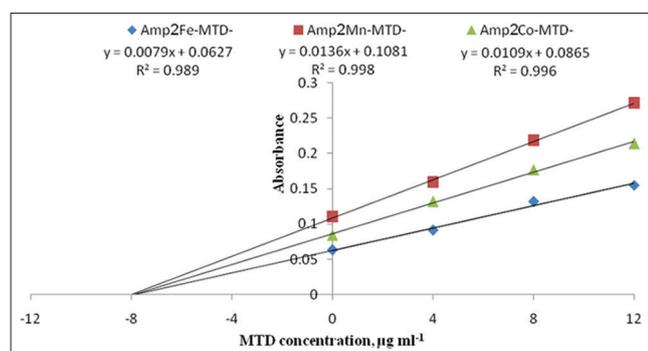
Fig. 8: Standard additions method for assay of Aldomet
