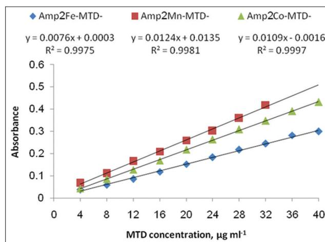
Fig. 6: Calibration graphs of the suggested systems
