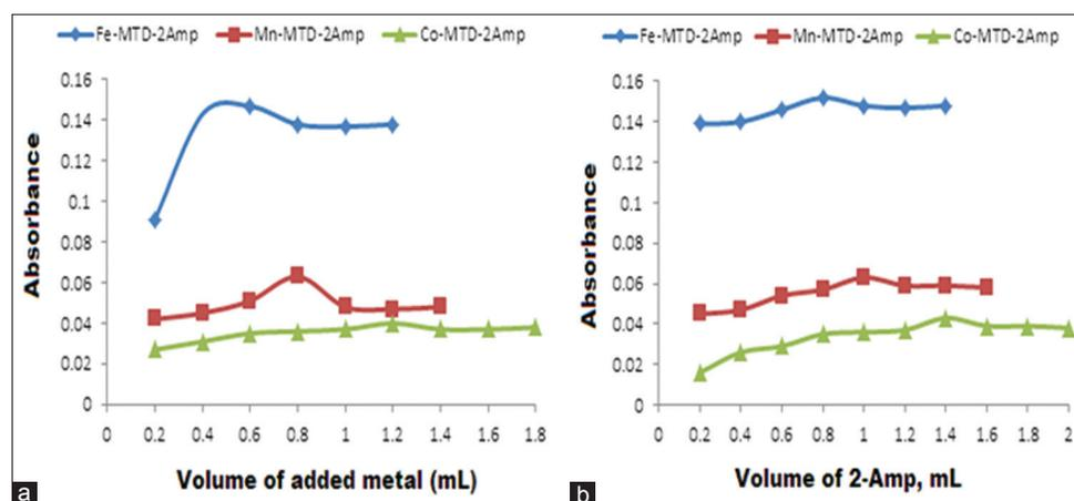
Fig. 2: (a and b) Selection of the suitable volumes of reacting reagent 2-aminopyridine and the added metal ion
