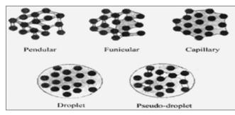
Fig. 1: Different formal spatial structures of liquid-bound agglomerates depending on liquid saturation
