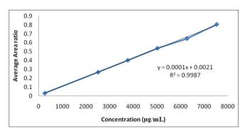
Fig. 5: Linearity graph of isopropyl alcohol
