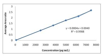
Fig. 4: Linearity graph of acetone
