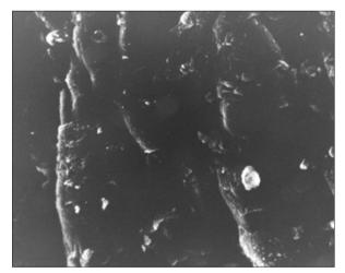
Fig. 2: Scanning electron microscopy image showing bioflexi film after release
