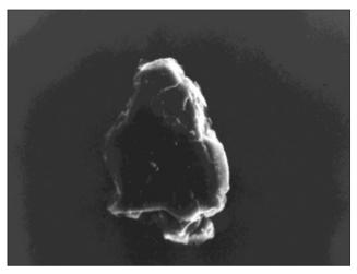
Fig. 1: Scanning electron microscopy image showing risperidone drug particle in bioflexi film
