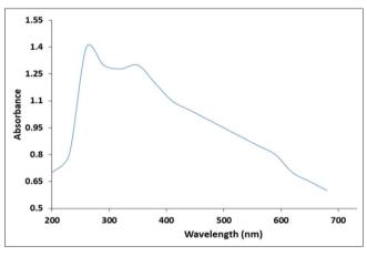
Fig. 1: Ultraviolet-visible spectroscopy of copper oxide nanoparticles
