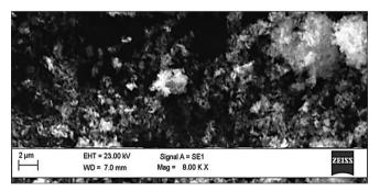
Fig. 2: Scanning electron microscopy images of copper oxide nanoparticles
