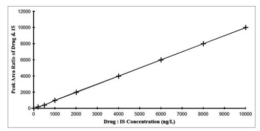
Fig. 1: Calibration curve of the paroxetine in blank human plasma using fluoxetine as internal standard in MRM mode (Y=1.004X+0.0045, R<sup>2</sup>=0.999)
