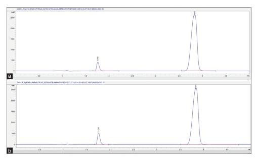
Fig. 4: (a) Chromatogram of standard amlodipine and telmisartan, (b) chromatogram of amlodipine and telmisartan in the formulation
