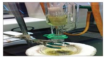
Fig. 3: Soxhlet extractor of plant
