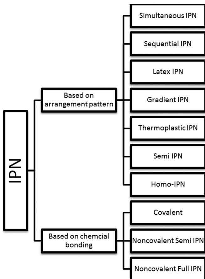
Fig. 2: Different forms of interpenetrating polymer network
