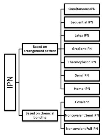
Fig. 2: Different forms of interpenetrating polymer network
