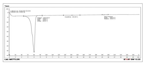
Fig. 2: Differential scanning calorimetry thermogram of sunflower wax
