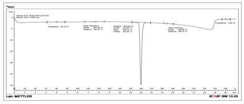
Fig. 1: Differential scanning calorimetry thermogram of salicylic acid
